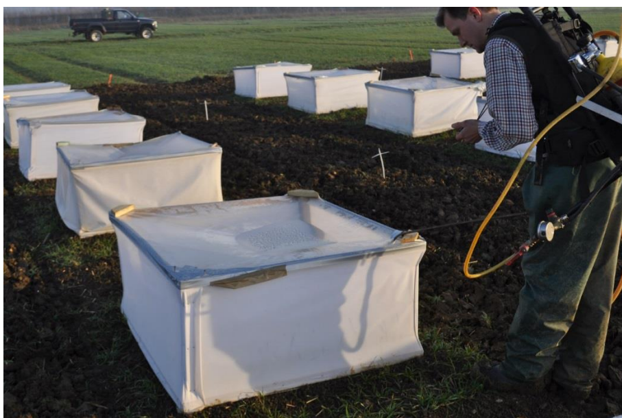
Figure 6. Wood-framed tents with breathable fabric sides and waterproof polyurethane top, ADAS Boxworth, February 2014. Small opening in top cover is used for inoculation with Z. tritici spores and for irrigation purposes. Frames in 2015 had additional cross-pieces under top cover to reduce rain water collecting on top.
